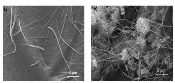
**Figure 3.** The surface morphology of (**a**) Di scaffold with 2 wt % MWCNTs; and (**b**) Di scaffold with 5 wt % MWCNTs.
