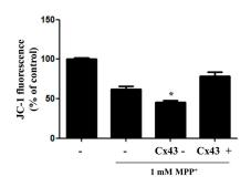
**Figure 3.** Overexpression of Cx43 inhibits MMP loss in MPP<sup>+</sup>-induced apoptosis. Cells were treated with 1 mM MPP<sup>+</sup>. MMP reduction was analyzed by JC-1 dye assay after 48 h of treatment with 1 mM MPP<sup>+</sup>. Cx43-: shRNA-Cx43, Cx43+: overexpression-Cx43; \* p < 0.05 compared with MPP<sup>+</sup>-treated group in one-way ANOVA followed by Bonferroni post hoc test.
