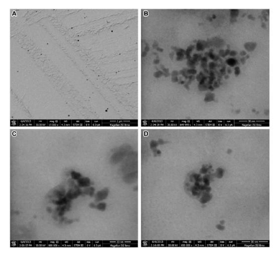
Figure S3. CdO nanoparticles in electron microscope (A–D).
