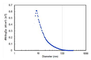
**Figure S1.** The size distribution of CdO nanoparticles in the size range 7.64–229.6 nm (measured in inhalled air with the SMPS, model 3936L72).
