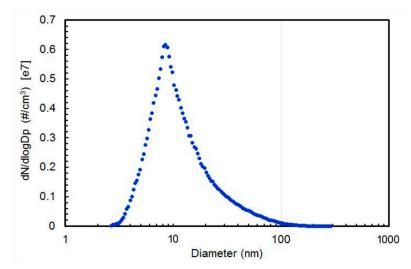
**Figure S2.** The combined size distribution of CdO nanoparticles in the size range 2.02–229.6 nm (measured in inhalled air with the SMPS, DMA model 3081 + nanoDMA model 3085).
