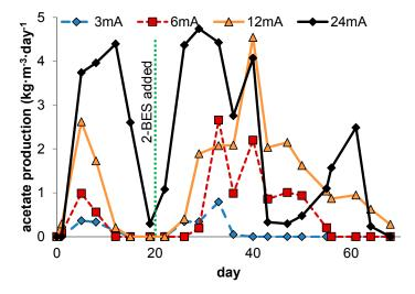
**Figure S3.** Acetate production rates as measured throughout the extended runs of the 4 current densities tested during the current controlled experiments. The green dotted line indicates the moment the systems were spiked with 10 mM of the methanogen inhibiting compound 2-bromoethanosulfonic acid (2-BESA).
