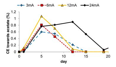
**Figure S2.** Acetate productions of the 4 different current densities tested during the current controlled experiments, with acetate production expressed as Coulombic efficiency (%), so normalized to the applied current.
