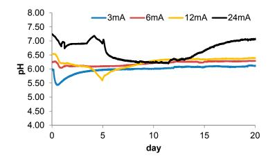
Figure S1. pH profiles of the 4 different current densities tested during the current controlled experiments.
