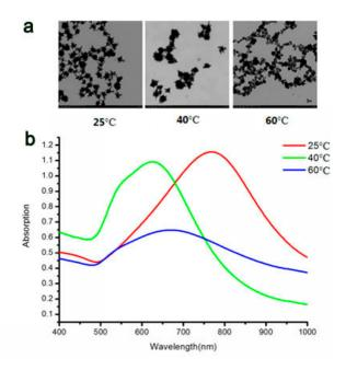
**Figure S1.** (a) TEM images and (b) UV absorption spectra of gold nanostars (GNS) with different reaction temperature (25 °C, 40 °C, and 60 °C).
