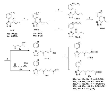
Scheme 2. Syntheses of 16a–e. Reagents and conditions: (a) BBr<sub>3</sub>, CH<sub>2</sub>Cl<sub>2</sub>, -78°C - RT; (b) CH<sub>3</sub>SO<sub>2</sub>Cl, Et<sub>3</sub>N, ethyl acetate, 0 °C; (c) CF<sub>3</sub>CH<sub>2</sub>OTf, K<sub>2</sub>CO<sub>3</sub>, DMF, RT; (d) DIBAL-H, CH<sub>2</sub>Cl<sub>2</sub>, -78 °C; (e) STAB, DCE, RT; (f) HCl/EtOH, RT.
