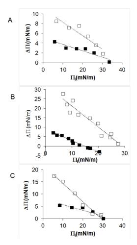
**Figure S7.** Surface pressure increase at equilibrium as a function of the initial surface pressure Pi) of the lipid monolayers induced by CitA (white squares) or CitO (black squares) adsorption. (**A**) PLPC, (**B**) Sitosterol, (**C**) PLPC/sitosterol (80/20) monolayer. Each point was obtained from an independent experiment.
