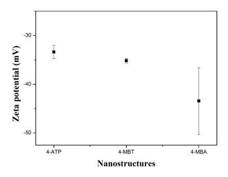
Figure S2. Zeta potential of SiO2@Au, SiO2@Au@4-ATP, SiO2@Au@4-MBT and SiO2@Au@4-MBA.
