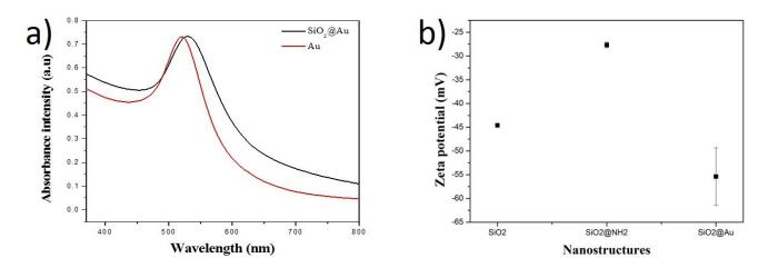
**Figure S1.** (a) UV-Vis of Au and SiO<sub>2</sub>@Au and (b) zeta potential of silica nanoparticles (SiO<sub>2</sub>), 3aminopropyltriethoxysilane (APTS) coated silica nanoparticles (SiO<sub>2</sub>@NH<sub>2</sub>) and gold embedded silica nanoparticles (SiO<sub>2</sub>@Au).
