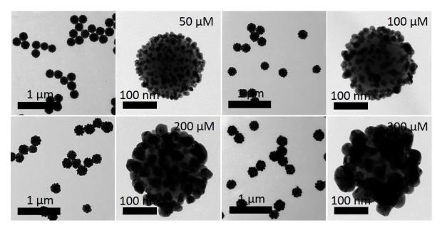
Figure S5. TEM images of SiO<sub>2</sub>@Au@4-MBT@Ag nanoparticles coated with different concentrations of AgNO<sub>3</sub>. Concentration of 4-MBT was 1 mM.
