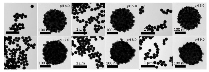
Figure S7. TEM images of SiO<sub>2</sub>@Au@4-ATP@Ag nanoparticles coated at different pH. Concentration of 4-ATP was 1 mM.
