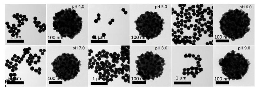
Figure S8. TEM images of SiO<sub>2</sub>@Au@4-MBA@Ag nanoparticles coated at different pH. Concentration of 4-MBA was 1 mM.
