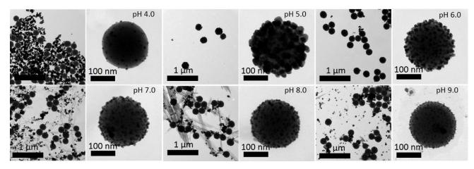
Figure S6. TEM images of SiO<sub>2</sub>@Au@4-MBT@Ag nanoparticles coated at different pH. Concentration of 4-MBT was 1 mM.
