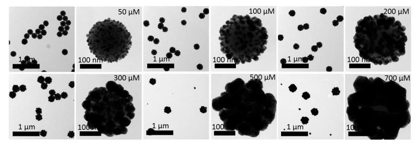
**Figure S3.** Transmission electron microscopy (TEM) images of SiO<sub>2</sub>@Au-4-MBA@Ag nanoparticles coated with different concentrations of AgNO<sub>3</sub> in water. Concentration of 4-MBA was 1 mM.
