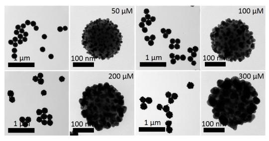
Figure S4. TEM images of SiO<sub>2</sub>@Au@4-ATP@Ag nanoparticles coated with different concentrations of AgNO<sub>3</sub>. Concentration of 4-ATP was 1 mM.
