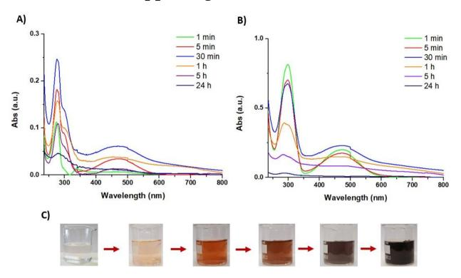
**Figure S1.** Evolution of the UV-vis absorption spectra of tyramine solutions (1 mM) (**A**) and dopamine solutions (**B**) during the enzymatic reaction in carbonate buffer at pH 6.8 over 24 h (diluted 10-fold before the measurement of the spectrum). (**C**) Digital pictures of catecholamine oxidation in the presence of 20 U/mL of tyrosinase.
