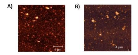
**Figure S3.** AFM image of a representative region of the  $\psi$ -PDA film sample, after 1 h of deposition onto the quartz crystal sensor, in the presence of 50 U/mL (**A**) and 100 U/mL (**B**) tyrosinase, respectively. Roughness: 28.7 nm (**A**), 12.8 nm (**B**). Film thickness: 63.3 ± 5 nm (**A**), 58 ± 4 nm (**B**).
