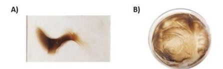
**Figure S7.** Calcium alginate hydrogel films on glass (**A**) or polystyrene (**B**) loaded with an 1% aqueous solution of tyrosinase and dipped into tyramine solution (1 mM) for 2 h.
