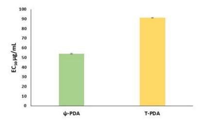
**Figure S5.** EC<sub>50</sub> values obtained from the DPPH assay of the samples obtained by oxidation of tyramine and dopamine in the presence of 20 U/mL of tyrosinase (2 mg/mL). The average values  $\pm$  SD obtained from at least three separate experiments are reported.
