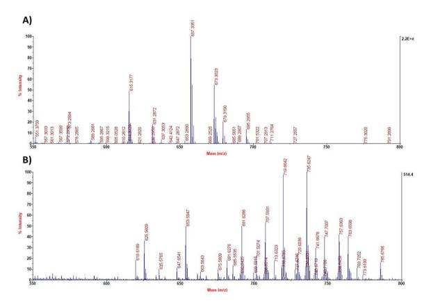
**Figure S4.** Segmental spectra of MALDI-ToF (m/z: 550–800 Da) characterizations of (**A**) tyramine film in carbonate buffer at pH = 6.8 with 20 U/mL of tyrosinase and (**B**) PDA film obtained under the same conditions.
