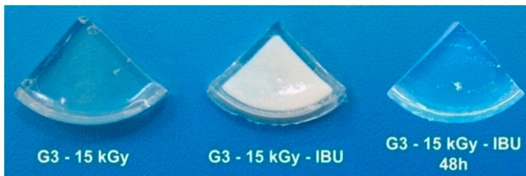
**Figure 11.** Picture of hydrogels obtained upon irradiation at 15 kGy, after encapsulation with ibuprofen (IBU) and respectively after complete drug release.
