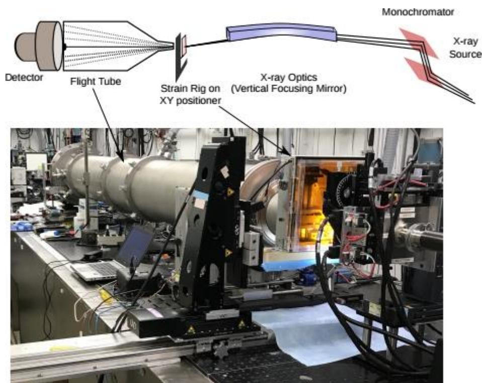
**Figure S4.** The schematic and a photograph of the XRD setup at BioCAT. The lower panel shows position of the sample strain rig positioned in the beamline for X-ray data collection.
