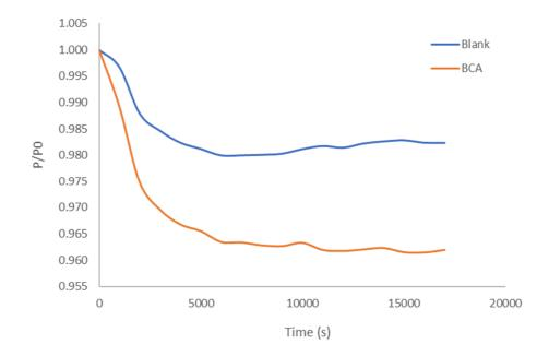
**Figure S3:** Time courses of pressure decay (normalized to the initial pressure – P<sub>0</sub>) as a function of time, during CO<sub>2</sub> sorption tests under pH 10. Raw data are plotted after using a smoothing tool, to minimize noise.
