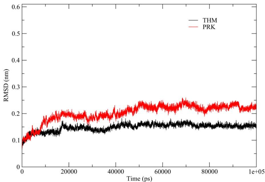
**Figure S1.** Time evolutions of the backbone RMSD values of the THM (black line) and PRK (red line) with respect to their starting structures during MD simulations at 300K.
