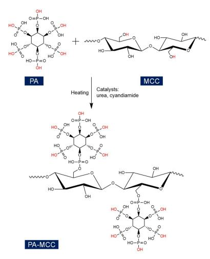
Figure 1. Schematic diagram of the preparation of PA modified MCC.
