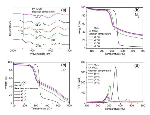
**Figure 4.** FT-IR (a), TG (b,c), and PCFC (d) analyses of PA-MCC obtained at various reaction temperatures. (PA concentration: 50%; MCC/PA weight ratio: 1:3; PA/urea/dicyandiamide weight ratio: 15:1:2; reaction temperature: 85, 90, 94 and 96  $^{\circ}$ C; 4 h).
