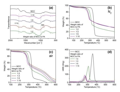
**Figure 3.** FT-IR (**a**), TG (**b**,**c**), and PCFC (**d**) analyses of PA-MCC obtained at various weight ratios of PA to MCC. (PA concentration: 50%; MCC/PA weight ratio: 1:2, 1:3, 1:5, and 1:10; PA/urea/dicyandiamide weight ratio: 15:1:2; 90 °C; 4 h).
