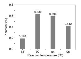
Figure 5. P content of PA-MCC obtained at various reaction temperatures.
