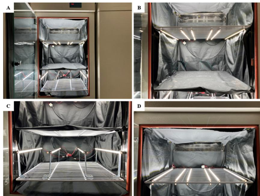
**Figure 9.** The plant growth chamber used in the study (A) and the light-emitting diode (LED) installed from the top (B), side (C), and bottom (D) relative to the plants.
