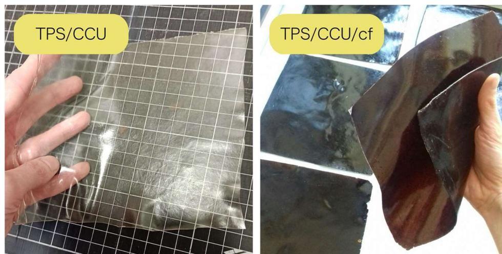
**Scheme 1.** Thermoplastic corn starch plasticized with CCU without filler (left) and with addition of spent coffee grounds (cf) (right).
