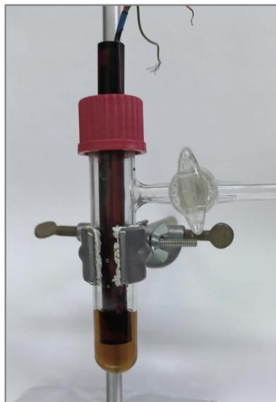
**Figure 13.** The electrochemical cell: the combined electrode rod is embedded in the polymer electrolyte solution. Removing the plasticizer (ethanol) was carried out by dipping the cell in an oil bath under vacuum. Cooling the solution was accomplished by dipping the cell in a cooling bath mixture composed of dry ice and organic solvent.
