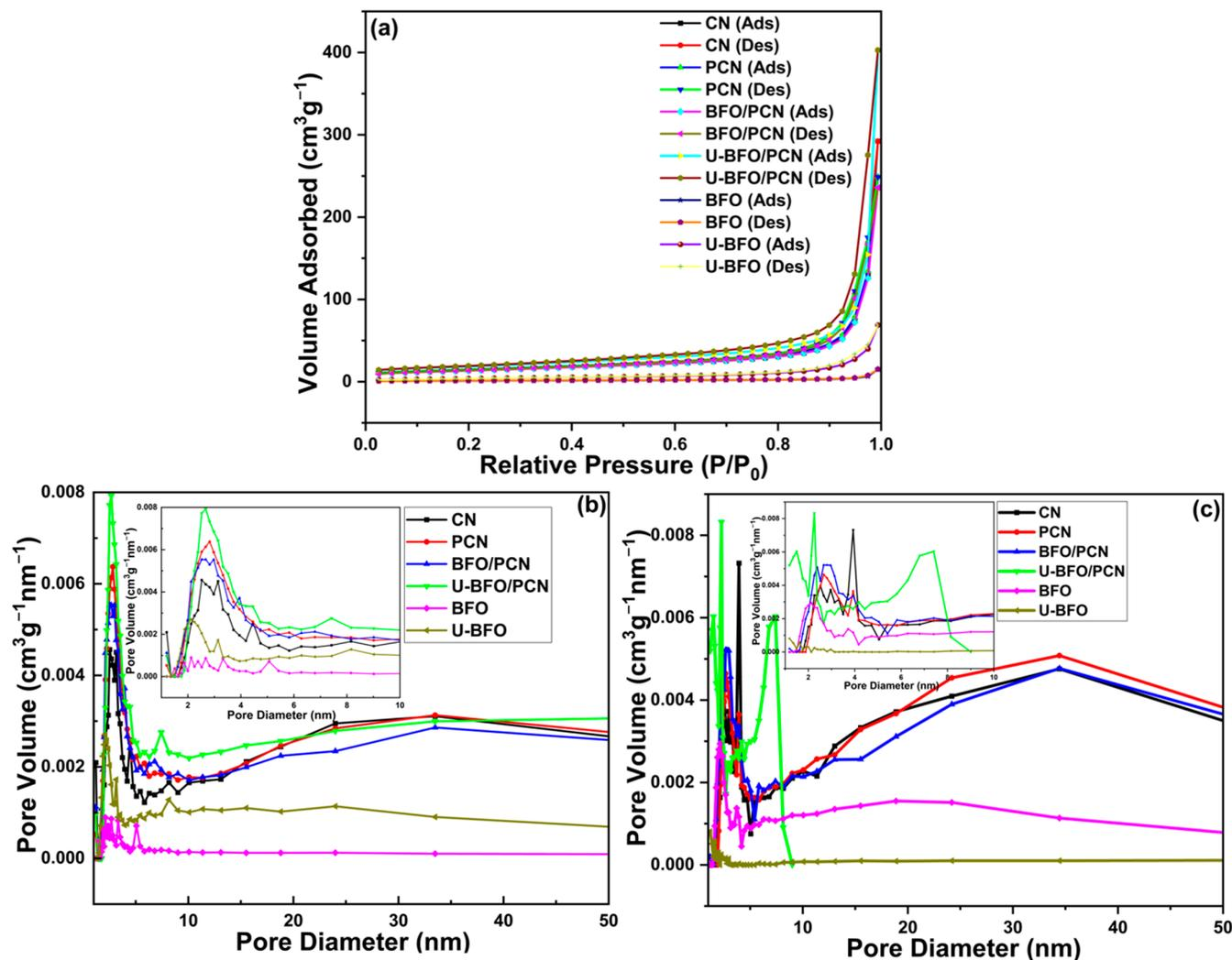
Figure 3. (a) N<sub>2</sub> adsorption–desorption isotherms and BJH pore size distributions for (b) adsorption and (c) desorption curves of pristine and composite photocatalysts.
