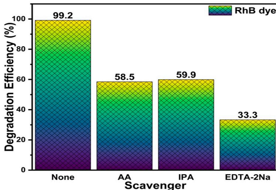
Figure 10. Scavenger tests for RhB degradation using U-BFO/PCN composites.
