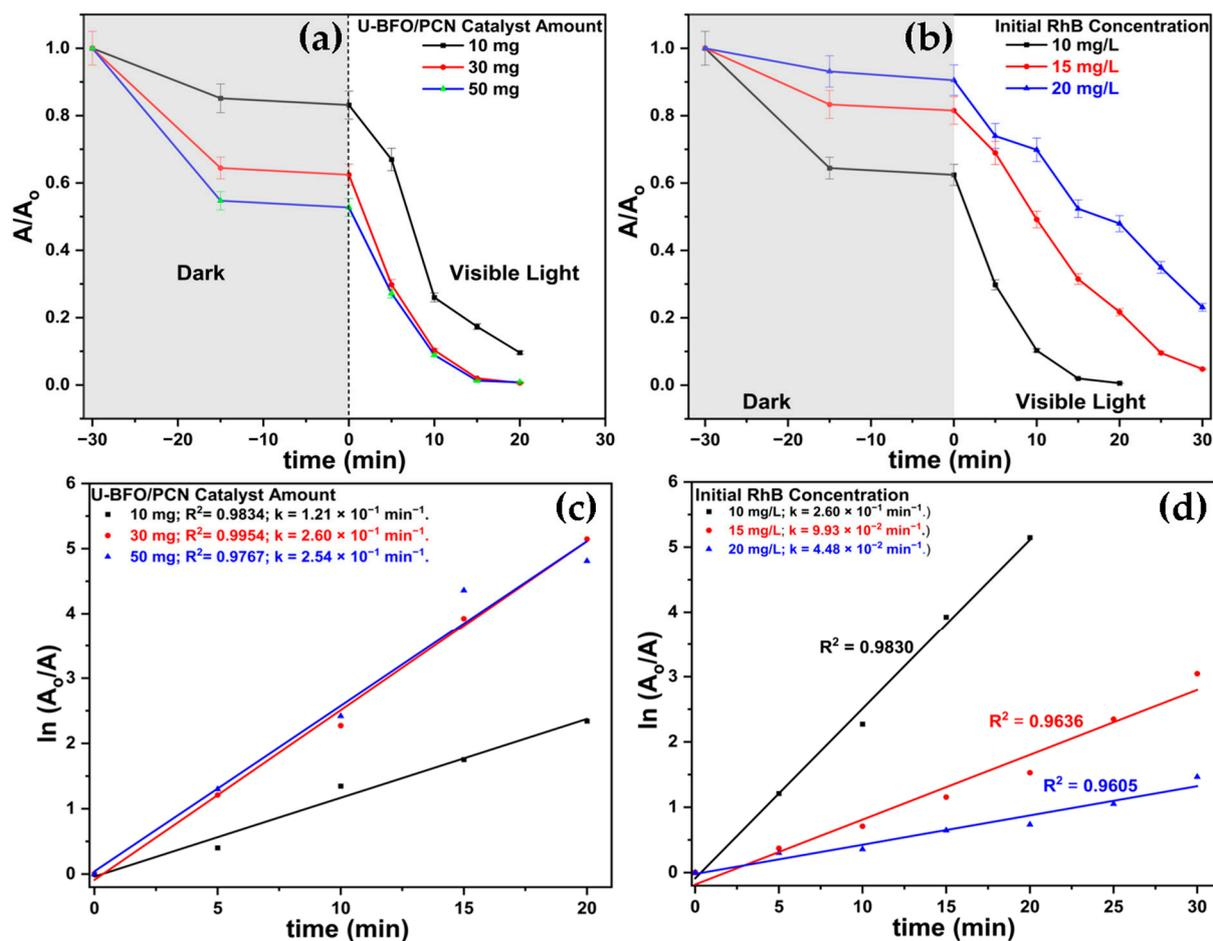
**Figure 9.** Photodegradation of varied amounts of U-BFO/PCN composites (a), varied initial RhB concentration (b), and their corresponding linearized pseudo-first-order plots (c,d).
