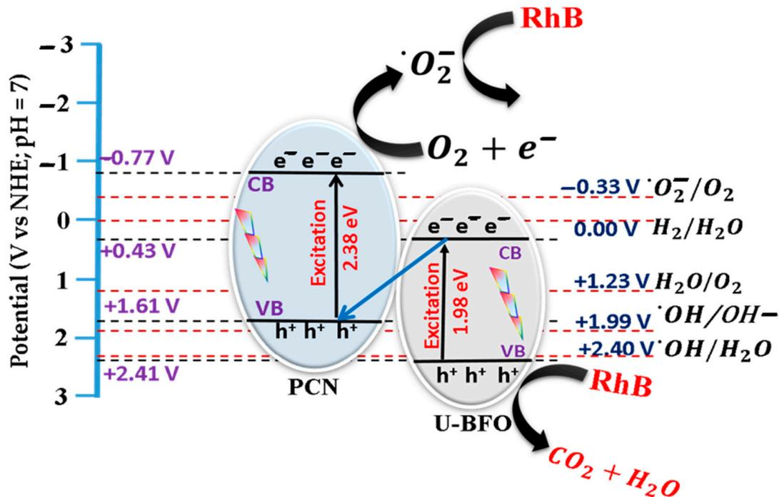
**Figure 11.** Proposed mechanism for RhB degradation over U-BFO/PCN heterojunction.
