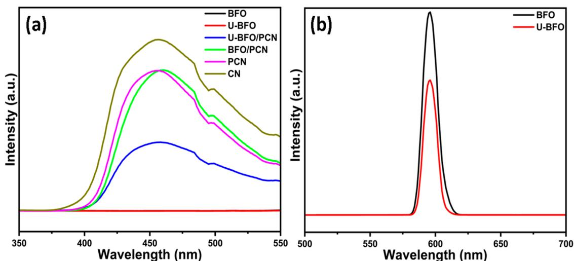
**Figure 7.** PL spectra (a) showing the emission of all the catalysts and (b) showing the emissions of BFO and U-BFO samples.
