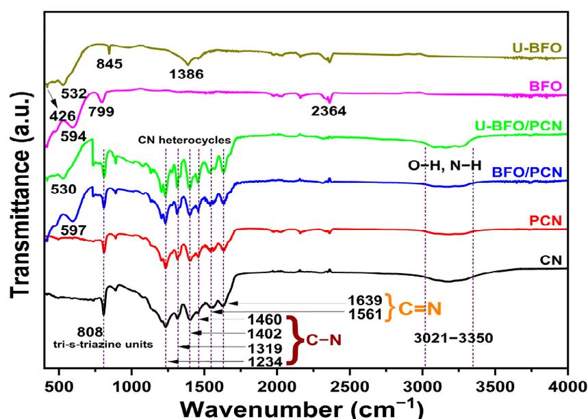
Figure 1. FT-IR spectral patterns of pristine and composite photocatalysts.
