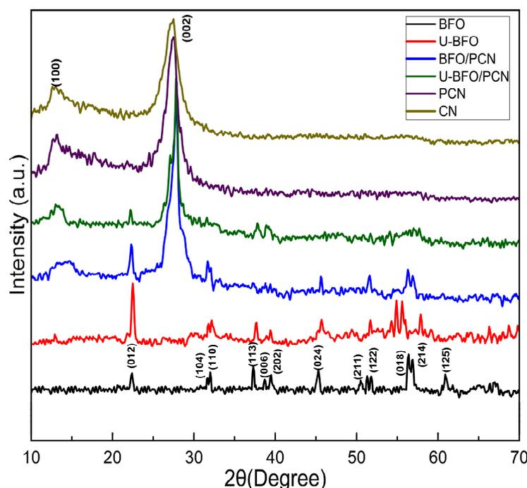
**Figure 2.** XRD patterns of pristine and composite photocatalysts.
