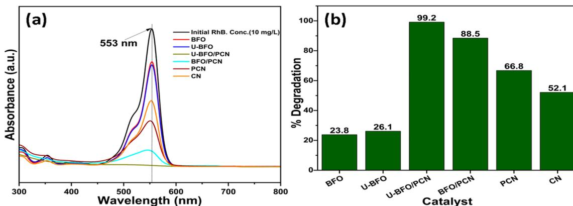
**Figure 8.** Absorbance spectra (a) and degradation efficiencies (b) of the pure and composite catalysts after 20 min of photodegradation.
