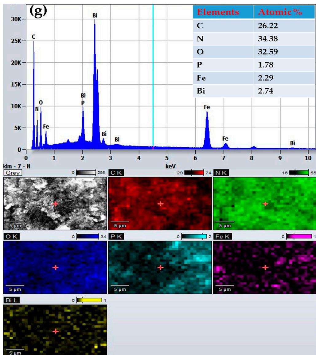
**Figure 4.** SEM images of (a) CN, (b) PCN, (c) BFO, (d) BFO/PCN, (e) U-BFO, (f) U-BFO/PCN, and (g) EDS spectrum and elemental mappings of U-BFO/PCN samples.
