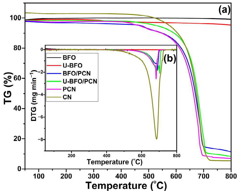
Figure 5. (a) TGA and (b) DTG curves of the pristine and composite samples.
