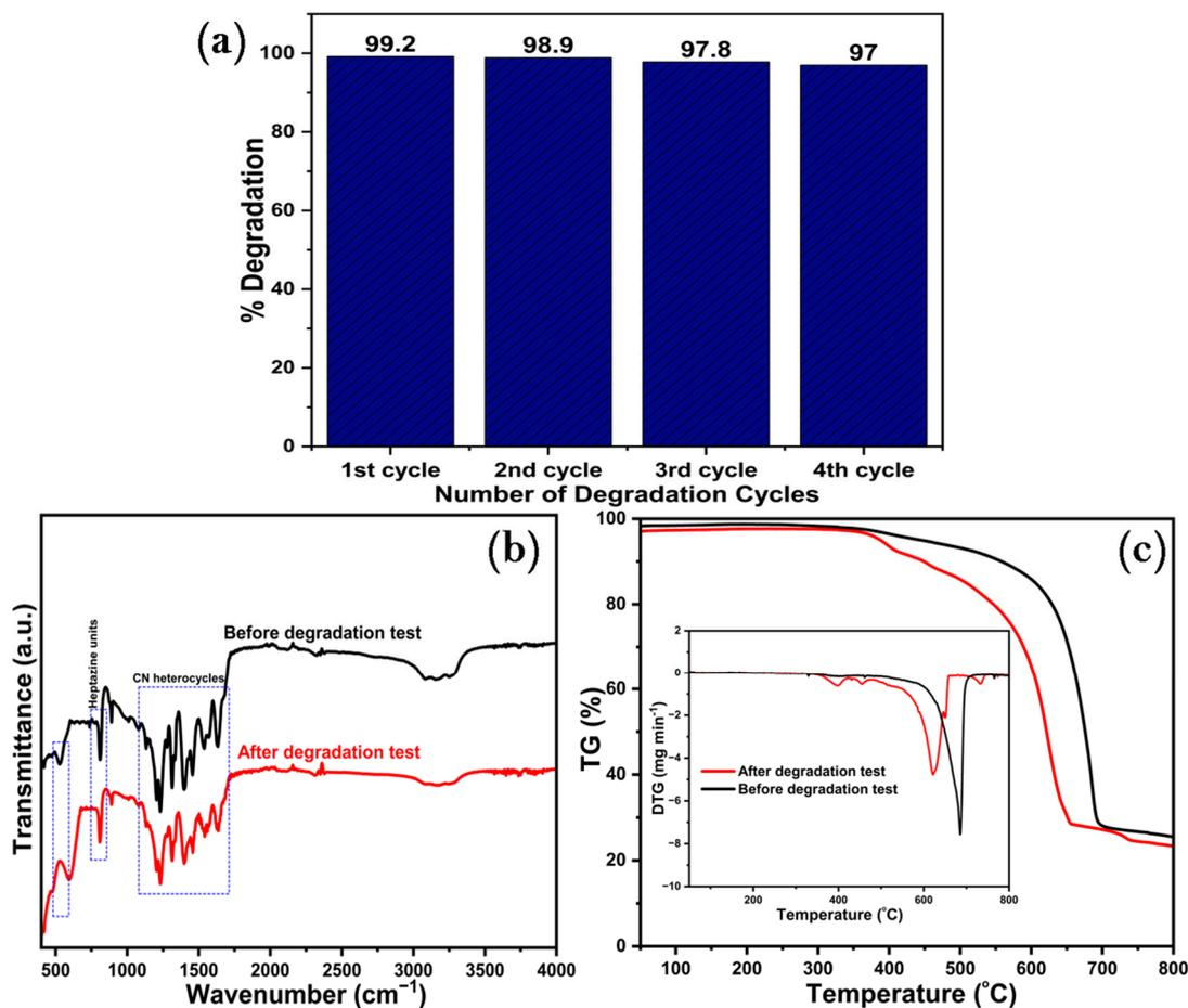
**Figure 12.** (a) Degradation runs (b) FT-IR spectra of U-BFO/PCN before and after the degradation experiment and (c) TG/DTG profiles of U-BFO/PCN before and after the degradation experiment.
