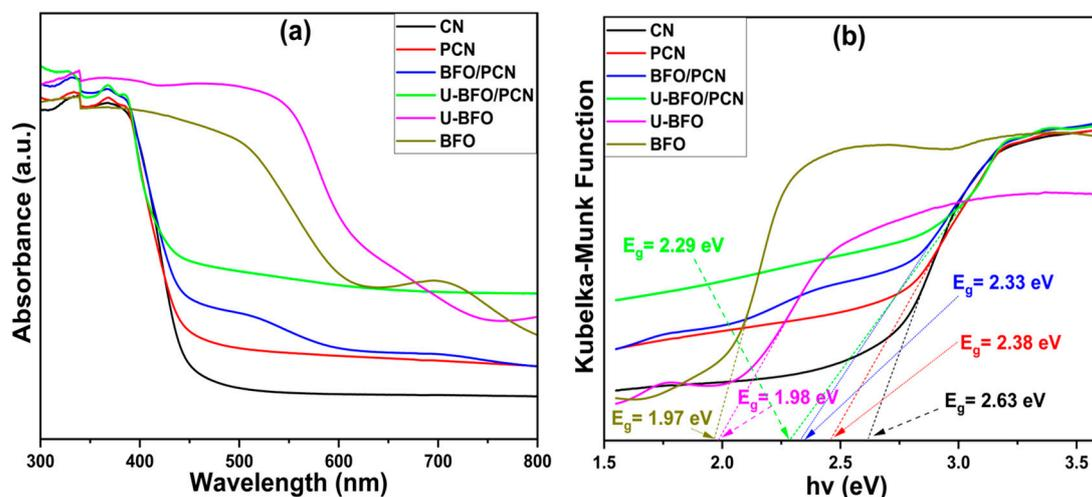
Figure 6. UV-vis spectra (a) and Tauc plot curves (b) of the pristine and composite samples.
