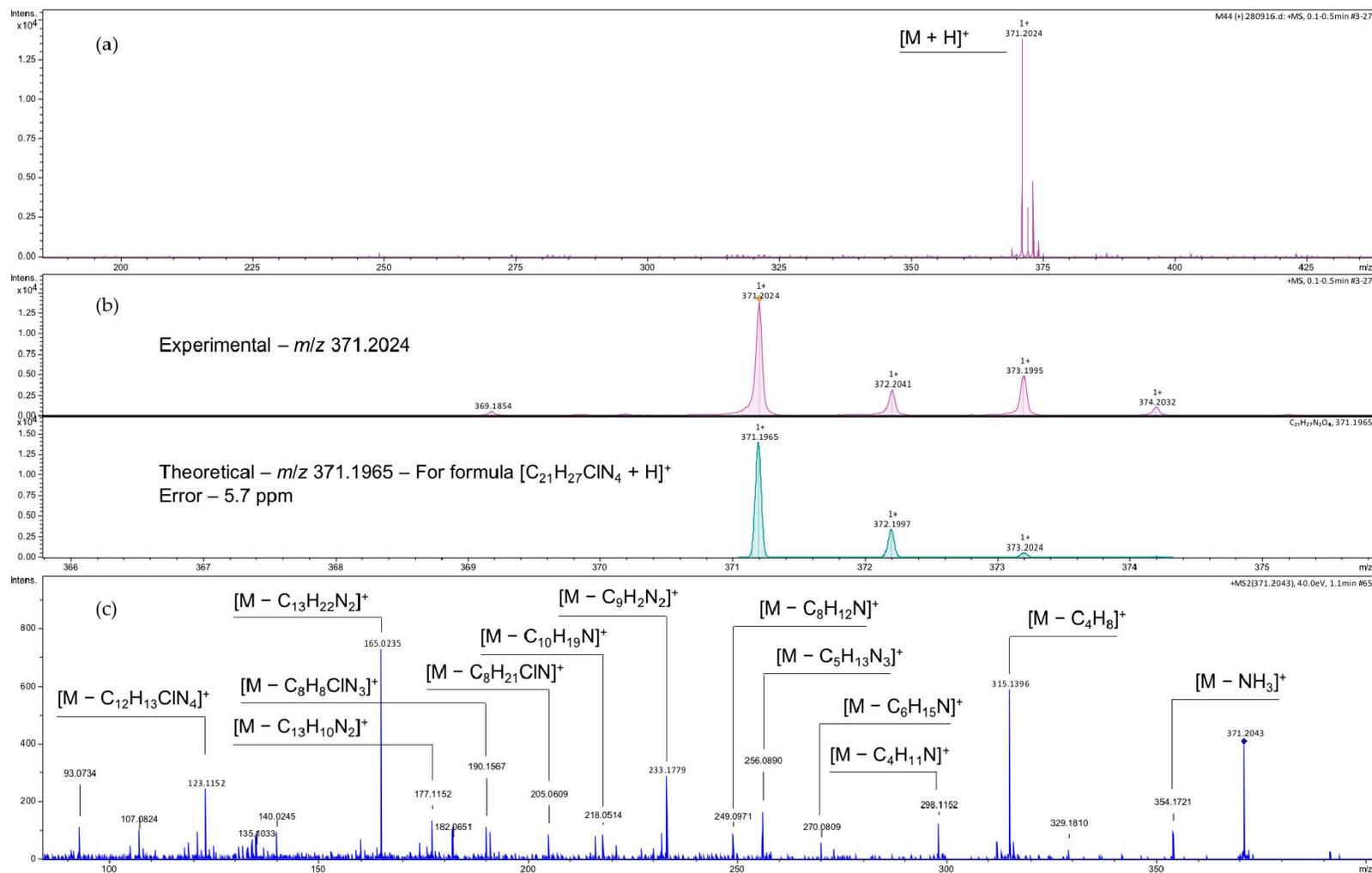
**Figure 1.** The HRMS analysis of compound 3. (a) the full spectra; (b) the expansion between 356 and 376 u.a.m. highlighting the exact mass and isotopic ratio; (c) the analysis in MS–MS mode (fragmentation pathway).
