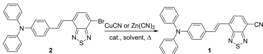
**Scheme 1.** Synthesis of (*E*)-7-(4-(diphenylamino)styryl)benzo[*c*][1,2,5]thiadiazole-4-carbonitrile **1**.
