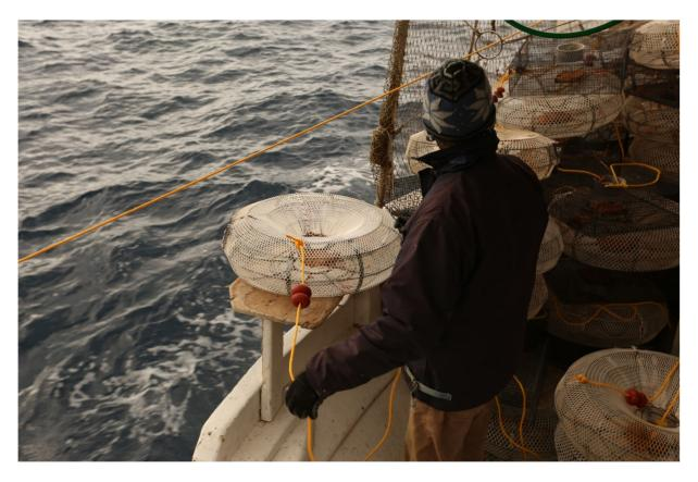
**Figure 2.** Commercial shrimp traps covered with polyamide-based nets of a mesh size of 12 mm (knot to knot) with an upper trap opening of 13 cm.
