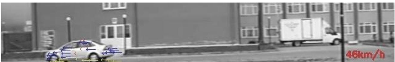
In Figure 1, the velocity vectors with the blue colour are error free correct vectors, yellow shows the velocity vectors of the shadow points and the red shows the mismatched point vectors. The image in the figure has been taken from a real experiment that we performed with our proposed system. The displacement amounts of all points (magnitudes of the vectors), which have been shown in the Figure 1 have been given in Table 4. The units of the displacements are in pixels.
