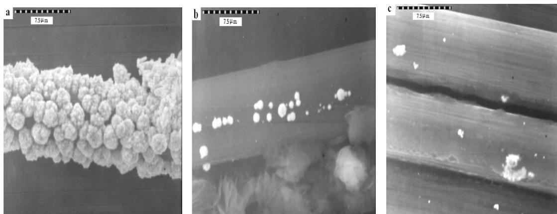
**Figure 11.** Gold particles distribution on a bundle of carbon fiber is composed of 8 single fiber and their lengths: (a) 6 cm; (b) 8 cm; (c) 12 cm.
