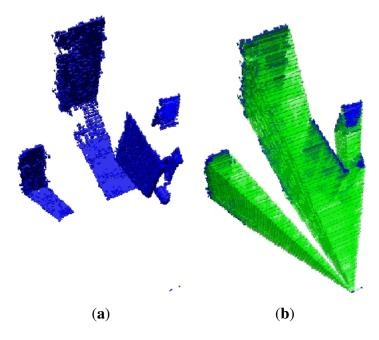
**Figure 11.** The obstacle is detected because it has been placed after the minimum range detection of the laser sensor.
