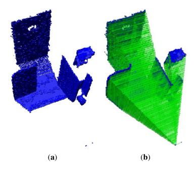
The second data set represents a 2D slide of the environment, which is represented as an occupied octree maps, shown in Figure 6(a), whereas Figure 6(b) shows the empty and occupied voxels. The main feature of this plot is the well-known wide field of view of the laser.
