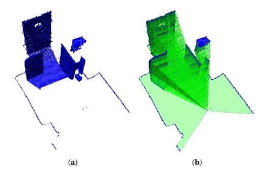
The laser octree data set representation is compared with the true map as shown in Figure 8. The walls, the objects, the corridor and the door are very well detected. This result just confirms the good accuracy tolerance of the current reading for most of the sensor's range.
