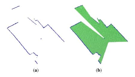
The fusion of the two previous data set readings is presented in Figure 12. The important fact to be noticed in this simulation result is that the laser really improves the minimum close range detection limitation of the Kinect<sub>TM</sub> sensor. In doing so, the robot can react and avoid an obstacle that is close and that is not detected by the Kinect<sub>TM</sub>, making the obstacle avoidance and hence the navigation safer and more reliable.
