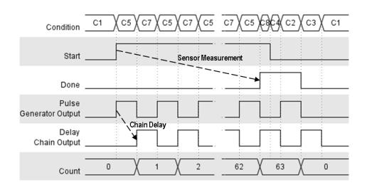
Figure 3. Chronogram of the main signals involved in the self-timed sensor.
