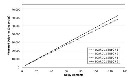
Figure 4. Constant-temperature sensor characterization.
