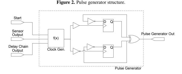
Timing equalization between the clock signals for both D-FFs is achieved by controlling the placement of all logic and memory elements involved. This can be achieved making use of the constraints supported by the FPGA vendor place&route (P&R) tools, a process which can be automated through configuration scripts.
