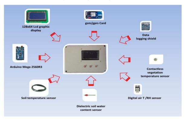
Figure 1. Components of platform.
