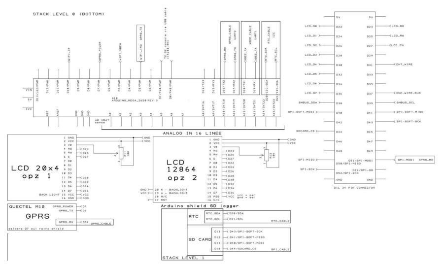
**Scheme 2.** Schematic electric diagram of sensors.
