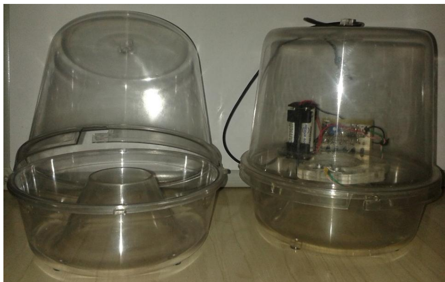
Figure 2. A typical plastic McPhail trap ( Left ) with the optoelectronic sensor embedded ( Right ).
