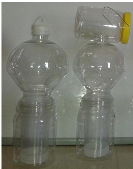
Figure 8. Traps used to capture alive B. oleae adults from olive trees. A typical olive-fly trap ( Left ); A custom-made trap with a second room attached ( Right ).
