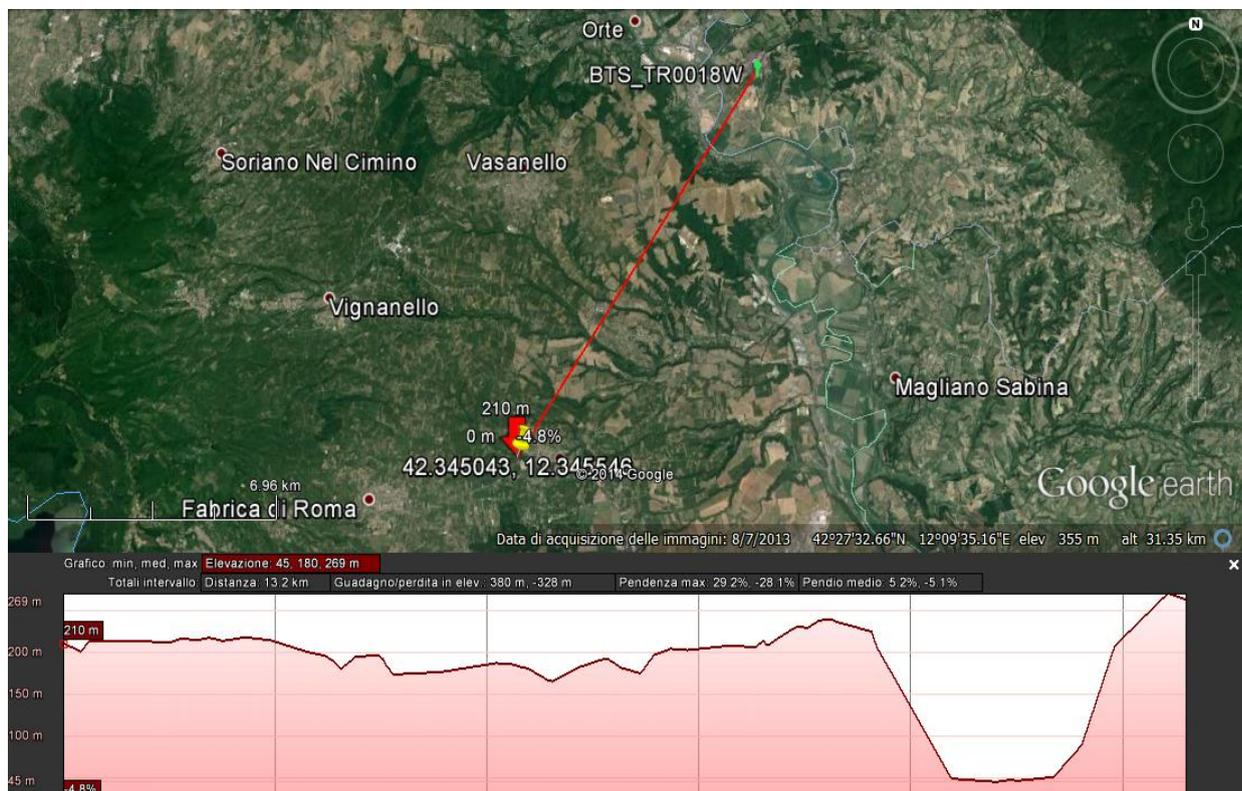
Even if the church is placed out of the WiMAX estimated cell edge, the WiMAX radio link has been successfully tested using the outdoors model HES-319M Customer Premise Equipment (CPE) [54]: the links have been correctly established with poor but stable radio parameters that can still guarantee a QPSK1/2 modulation in UpLink and QPSK3/4 in DownLink.
