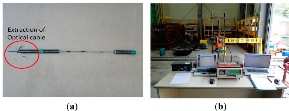
**Figure 4.** (a) Carbon core wire specimen for sensing strand and (b) setting of core wire test.
