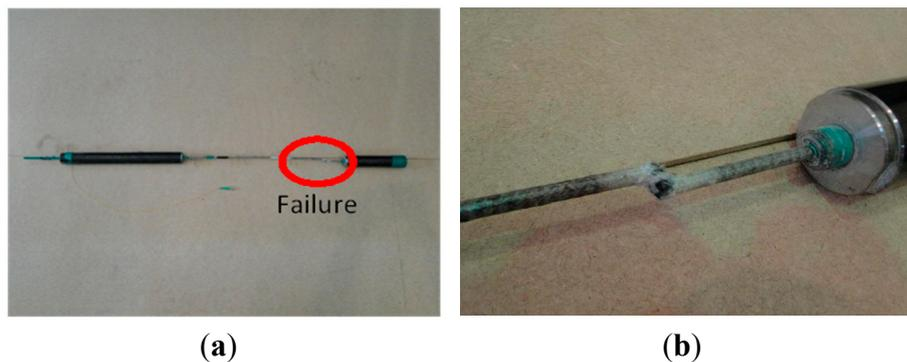
**Figure 6.** (a) Failure pattern of carbon core wire specimens and (b) detailed view.
