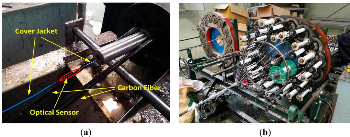
**Figure 2.** (a) Insertion of optical sensor and (b) fabrication of carbon core wire.
