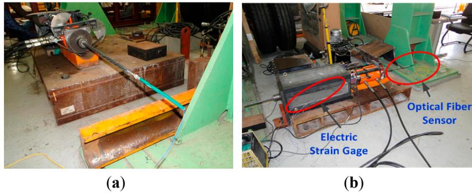
**Figure 5.** (a) Sensing strand specimen and (b) setting of strand performance test.
