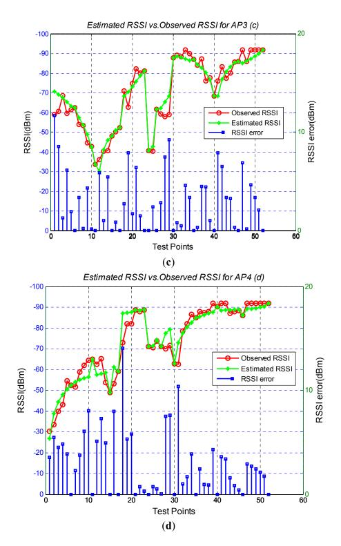
Figure 4. Estimated RSSI errors for testing points in scenario one. (a) Estimated Results for AP1; (b) Estimated Results for AP2; (c) Estimated Results for AP3; (d) Estimated Results for AP4
