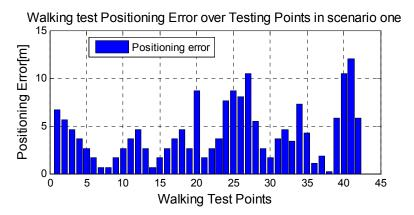
Figure 6. Walking Test positioning errors on Floor 12 with the proposed Radio map.
