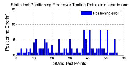
Figure 5. Static Test positioning errors in scenario one with the proposed radio map.
