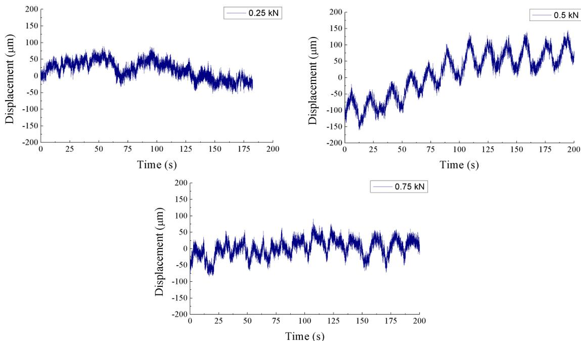
**Figure 9.** POE elongation corresponding to the three fatigue cycles of 0.25 kN, 0.5 kN and 0.75 kN.
