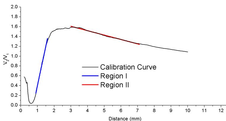
**Figure 18.** Calibration curve of the sensor showing the two possible regions of measurement: region I (front-slope) in blue and region II (back-slope) in red.
