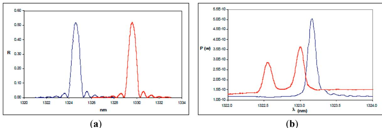
**Figure 2.** (a) Ideal behavior of the reflected spectrum of an FBG subjected to a longitudinal strain; (b) Effect of a transverse stress on the reflected spectrum of the FBG. In all figures the blue line represents the non-perturbed spectrum of the FBG and the red one is the spectrum after the application of the load.
