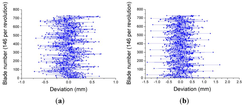
**Figure 23.** Deviation of each blade from the equilibrium position obtained four days later at 3390 rpm (a) and 5570 rpm (b).
