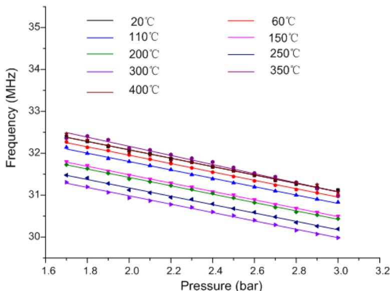
**Figure 11.** Measured curve of the pressure sensing element after temperature compensation.
