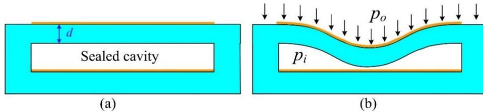
**Figure 7.** Pressure sensor model (a) before deformation (b) after deformation.
