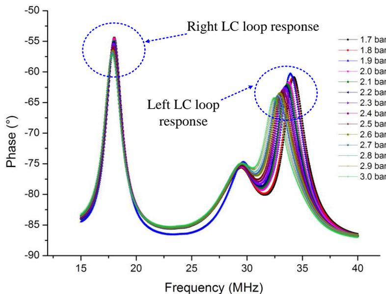
**Figure 10.** Proposed compensation structure pressure response in 200 °C.
