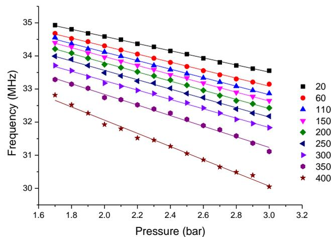
**Figure 6.** Extracted frequency versus pressure at different temperatures.
