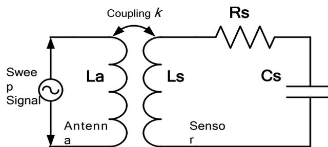
**Figure 3.** Equivalent measurement principle of the fabricated sensor.
