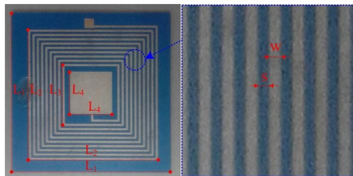
**Figure 2.** Fabricated pressure sensor.
