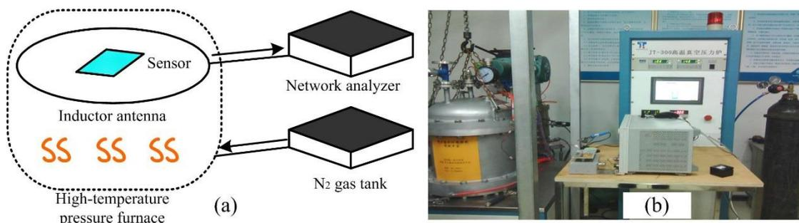
**Figure 4.** (a) Schematic and (b) physical diagrams of the high temperature/pressure complex measurement system.
