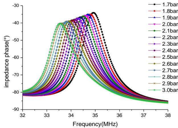
**Figure 5.** Readout signals of different gas pressures at 20 °C.
