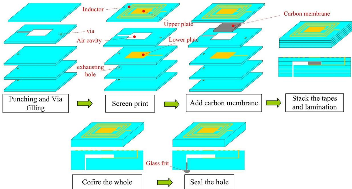
**Figure 1.** Main fabrication processes of the pressure sensor.
