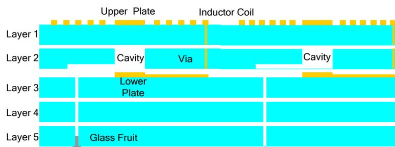
**Figure 9.** Temperature compensation structure for complex environments.
