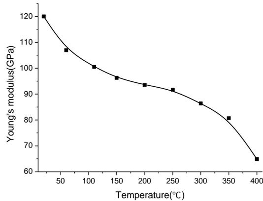
**Figure 8.** Calculated Young's modulus of LTCC at different temperatures.
