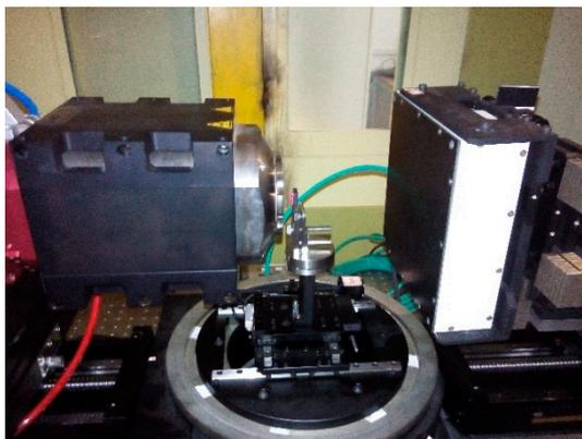
**Figure 5.** Photograph of the micro-CT system with a micro-focus X-ray source, rotation stage, and a flat panel detector.
