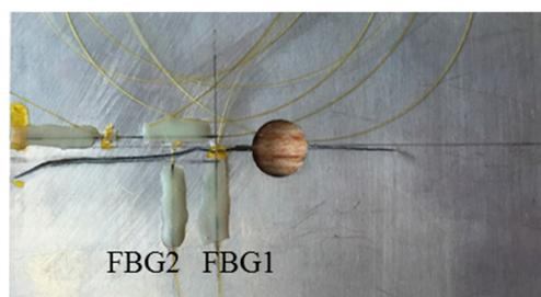
**Figure 13.** The crack propagation path observed in the experiment. Note the curved path of the crack which introduces additional error from the numerical model.
