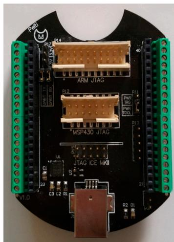
**Figure 47.** The PDL shield, named as Pelti, with JTAG connectors, USB connector, and screw-type terminal blocks connected to all of the S-BECs signals.
