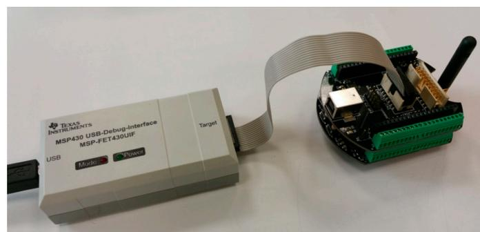
**Figure 48.** Programming and debugging setup using the MSP-FET430UIF tool from Texas Instruments. The PDL shield is connected onto the WNL shield through the S-BECs and J-BEC for easy access to the required JTAG signal pins.
