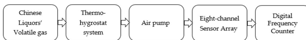
**Figure 7.** Working flow chart of the e-nose.
