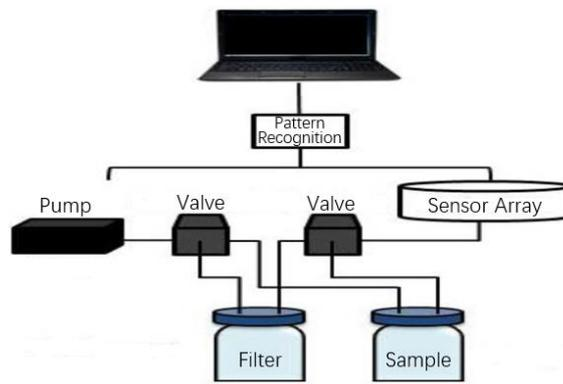
Figure 4. Schematic diagram of the QCM-based e-nose.
