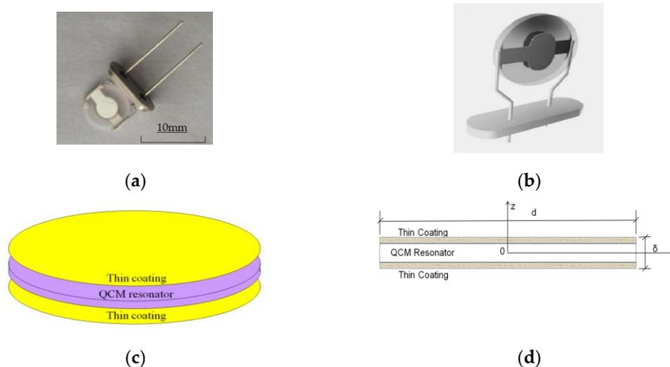
**Figure 1.** (a) Photo of the sensor; (b) structure chart of the sensor; (c) schematic diagram of the sensor; (d) diameter drawing of the sensor.
