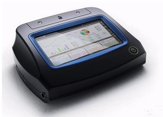
**Figure 3.** Photo of the QCM-based e-nose.
