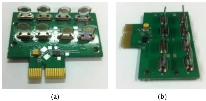
Figure 5. Image of the QCM sensor array. (a) front view; (b) side view.
