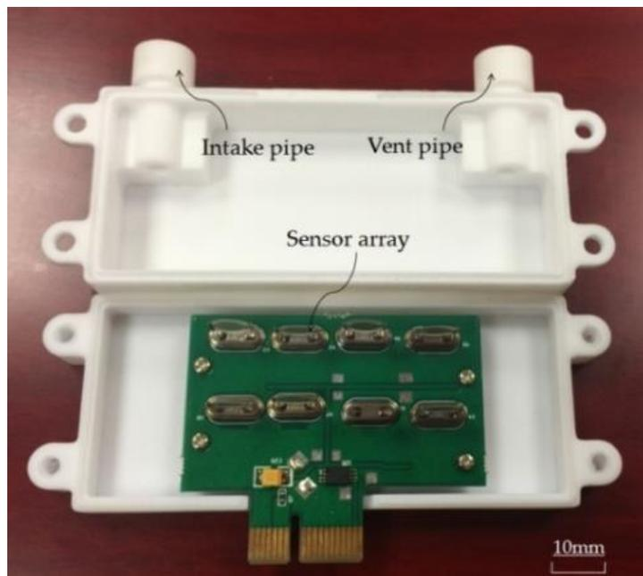
Figure 6. Photo of the sensor box.
