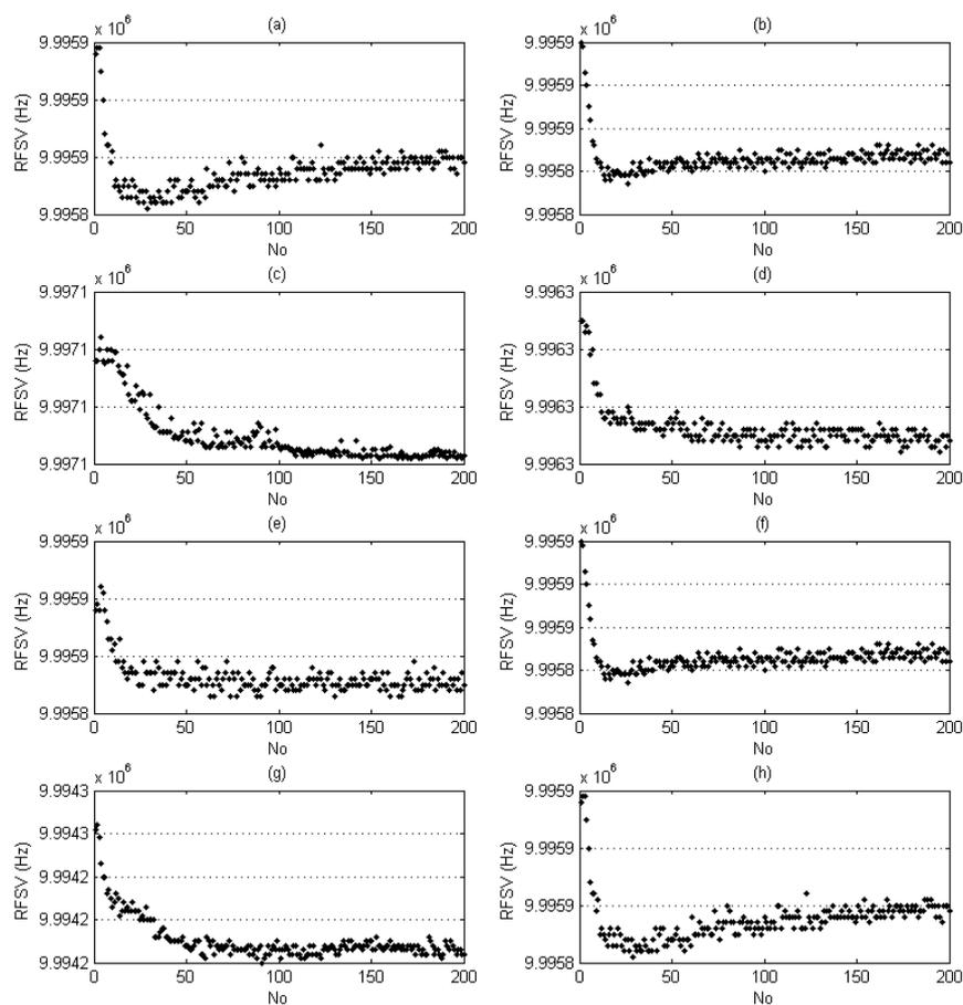
**Figure 8.** Group of raw data of the Moutai sample's characteristic information from Sensor-1 to Sensor-8: (a) Sensor-1; (b) Sensor-2; (c) Sensor-3; (d) Sensor-4; (e) Sensor-5; (f) Sensor-6; (g) Sensor-7; (h) Sensor-8.
