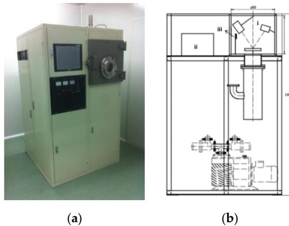
**Figure 2.** (a) Photo of the EBVD equipment; (b) schematic representation of the EBVD technology: (i) electron beam deposition system in vacuum chamber; (ii) control system; (iii) coating thickness control system.
