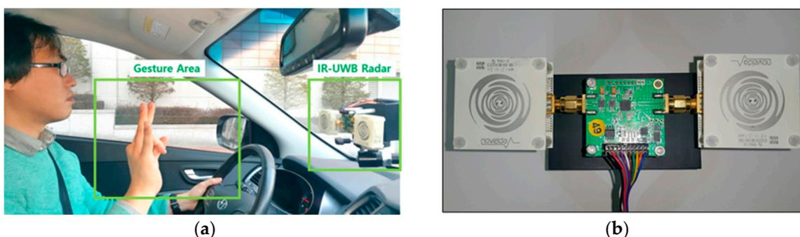
**Figure 13.** (a) Experimental setup inside the car; (b) IR-UWB radar.
