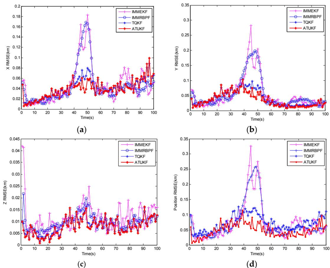
**Figure 5.** Root-mean-square error (RMSE) of the ATUKF, IMMEKF and IMMRBPF. (a) X RMSE; (b) Y RMSE; (c) Z RMSE; (d) position RMSE.
