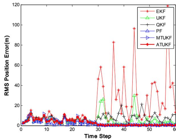
**Figure 2.** Root-mean-square (RMS) position errors of the extended Kalman filter (EKF), unscented Kalman filter (UKF), quadrature Kalman filtering (QKF), PF, mixture truncated unscented Kalman filter (MTUKF) and auxiliary truncated unscented Kalman filtering (ATUKF).
