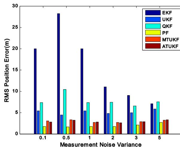
**Figure 3.** RMS position error for different noise variances.
