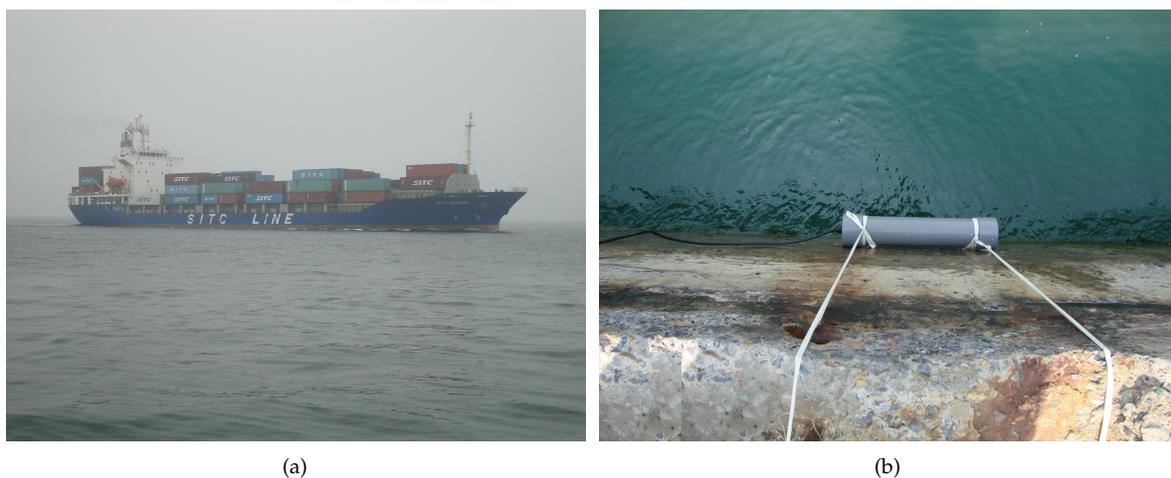
**Figure 2.** The detection experiment on a shallow sea. (a) the surface ship as the target; (b) the magnetic field sensor above the sea surface.
