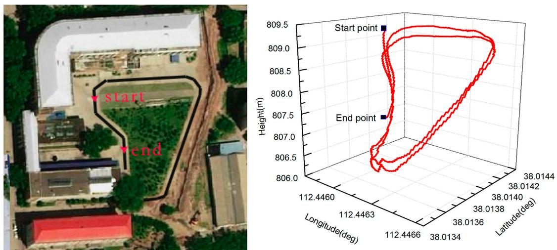
**Figure 9.** The reference trajectory of the vehicle. The two-dimensional reference trajectory of the vehicle (Left) and the corresponding three-dimensional trajectory (Right).
