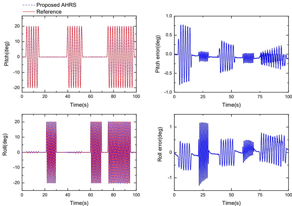
**Figure 13.** Orientation estimate produced by the proposed algorithm (left,  $\mu_a = 0.005$ ) and the difference between the estimate and reference (right).
