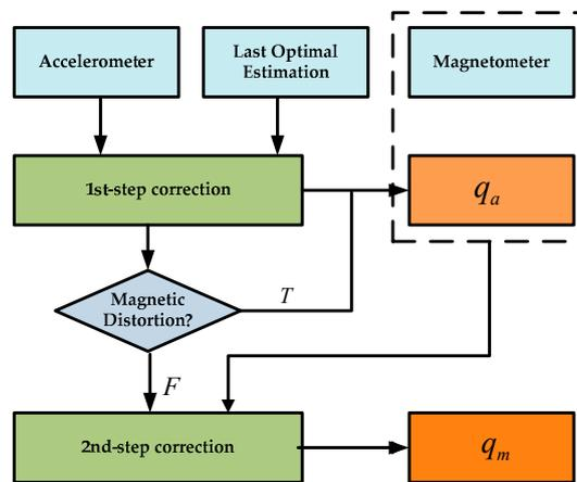
Figure 2. Block diagram of the TGIC.
