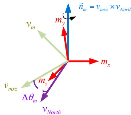
Figure 4. Correcting the estimated direction of the magnetic field using magnetometer.
