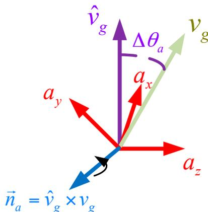
Figure 3. Correcting the estimated direction of gravity using the accelerometer.
