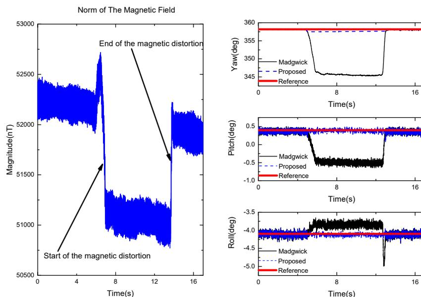
**Figure 15.** The norm of the magnetic field (left) and the orientation produced by the proposed algorithm (blue,  $\mu_a = 0.9$ ), Madgwick's complementary filter (black,  $\beta = 0.8$ ) (right).
