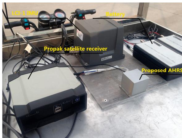
**Figure 8.** The vehicle test platform and designed AHRS used in this experiment.
