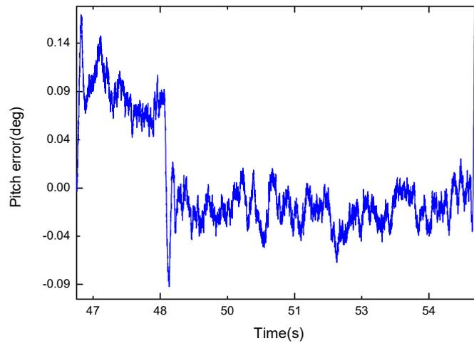
**Figure 12.** Difference between the pitch estimate and turntable reference.
