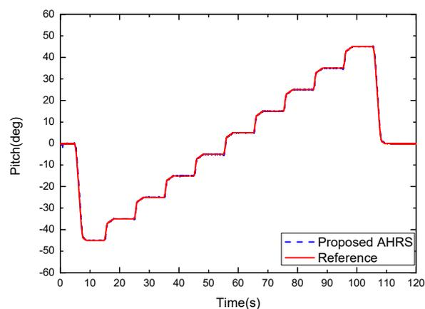
**Figure 10.** Pitch estimate produced by the proposed Kalman filter (blue dash curve,  $\mu_a = 0.9$ ) and the turntable reference (red solid curve).
