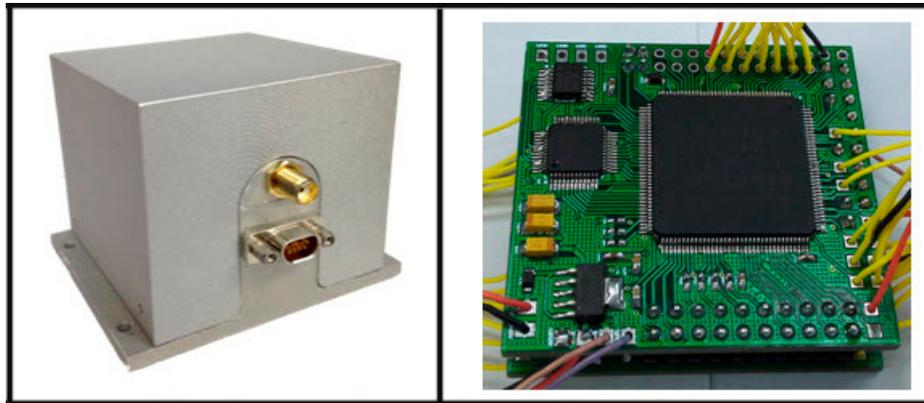
Figure 6. Homemade prototype of the AHRS. Homemade prototype of the AHRS (Left) and its circuit component (Right).
