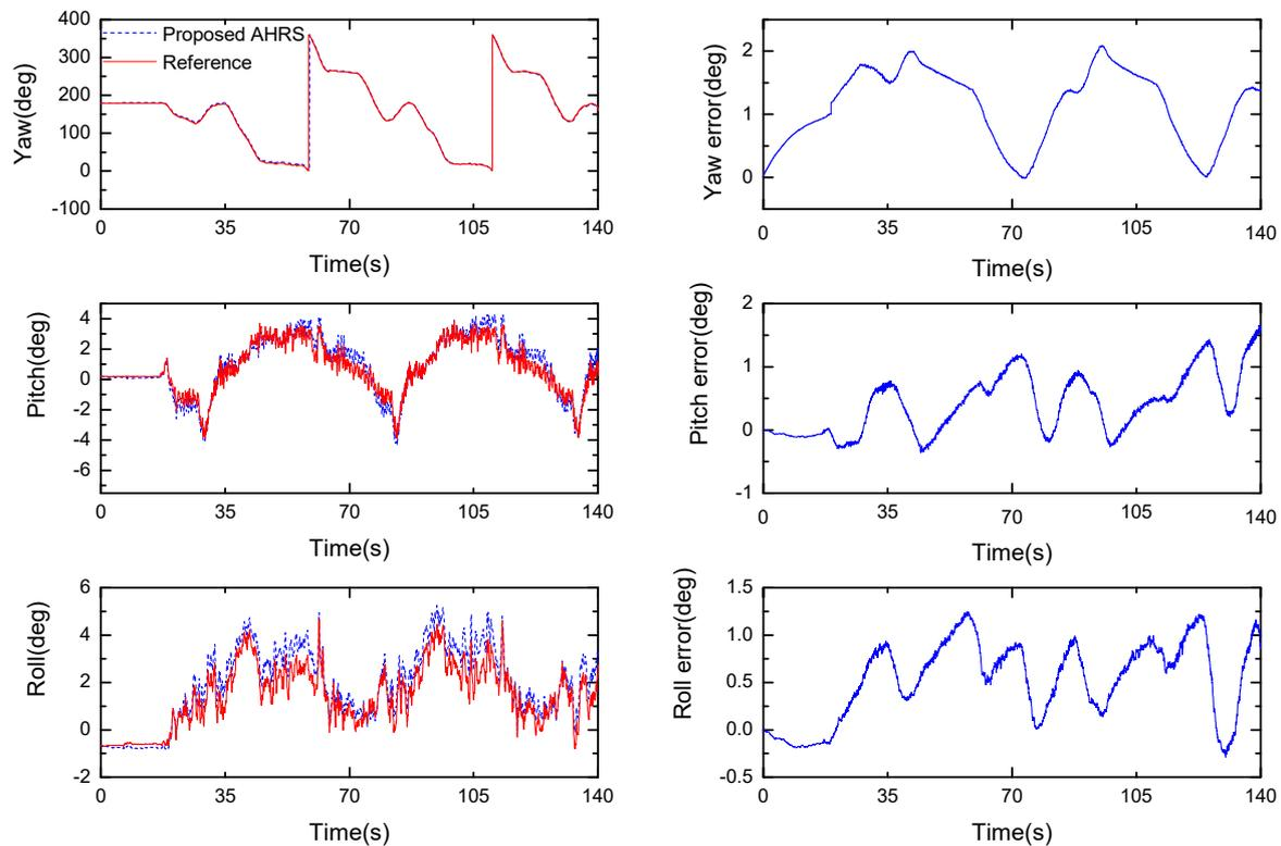
**Figure 14.** Orientation estimate produced by the proposed algorithm (left,  $\mu_a = 0.001$ ) and the difference between the estimate and reference (right).
