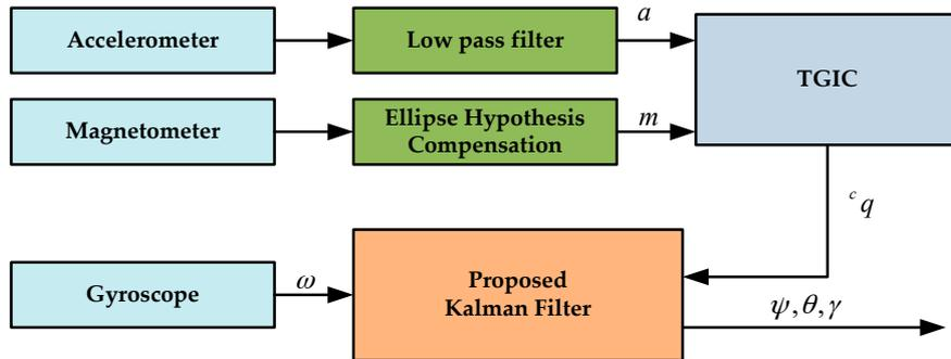
Figure 1. Block diagram of the proposed KF design.
