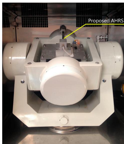
**Figure 7.** Physical map of three-axis turntable testing.
