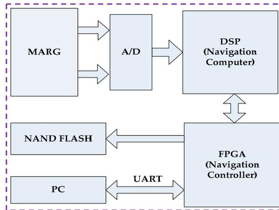
Figure 5. Structural diagram of the AHRS.
