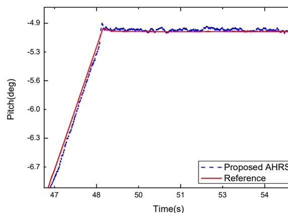
**Figure 11.** Zoomed-in view of the pitch estimate (dash curve) from the Kalman filter and the turntable reference (solid curve).
