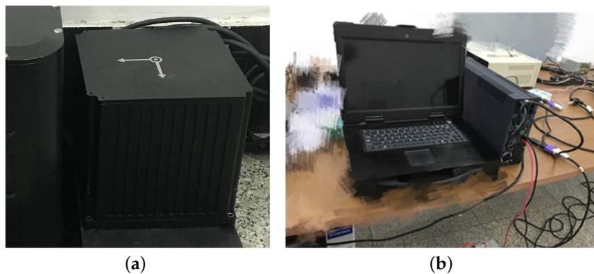
**Figure 4.** Static test in the laboratory. In this test, a FOG IMU, developed by the Navigation Instrument Institute, Harbin Institute of Technology, is used as shown in (a). This FOG IMU is placed on a stable and leveled marble platform to isolate the influence from external disturbance; In (b), a rugged laptop is used to collect the source data.
