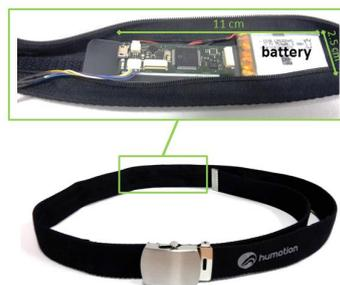
**Figure 4.** The sensor belt includes a 3D accelerometer, gyroscope and magnetometer, as well as a barometer.
