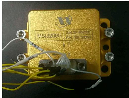
Figure 3. MSI3200 Inertial Measurement Unit.
