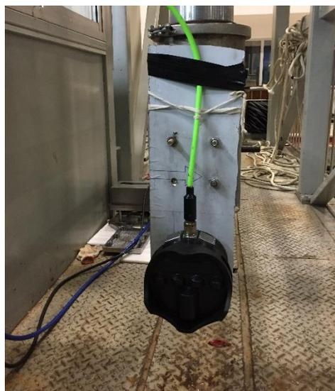
**Figure 10.** The Kongsberg M3 multibeam sonar and installation method for the experiment.
