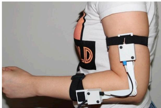
Figure 3. Positioning of the POF sensor at the elbow joint.
