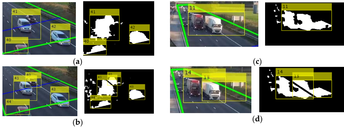
Figure 4. Occlusion handling when cases 1 and 2 are fulfilled, green lines indicate the ROI, and blue line the detection line. Actual image and foreground mask, (a,c) before applying the algorithm and (b,d) after applying the algorithm.
