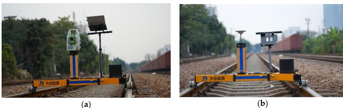
**Figure 8.** Modular design of the TGMT based on aided INS. (a) TGMT with TS/INS configuration; (b) TGMT with GNSS/INS configuration.
