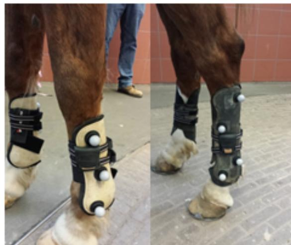
**Figure 9.** Placement of the IMU sensors and optical motion capture markers on fore- and hindlimbs.
