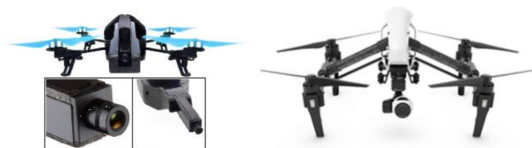
Figure 2. Commercial drones with on-board cameras: Parrot AR.Drone 2.0 (Parrot, Paris, France) (left) and DJI Inspire 1 (DJI, Shenzhen, China) (right).
