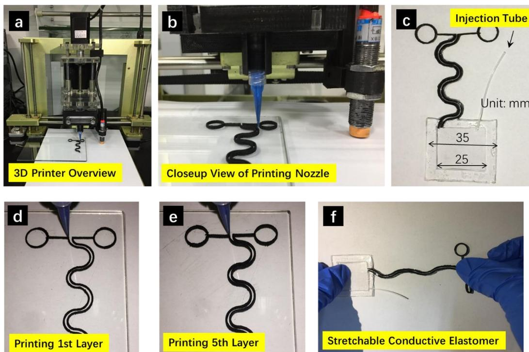
**Figure S2.** (a) Overview of the home-built 3D printer; (b) Close-up view of printing nozzle for extrusion of conductive CNT/PDMS ink; (c) Photograph of a complete pressure sensor with solution pool and injection tube; (d–e) Photographs of printing 1st layer and 5th layer of the elastomer electrode directly on temper glass substrate; (f) Photograph of the capillary electrodes made of conductive elastomer upon stretching.
