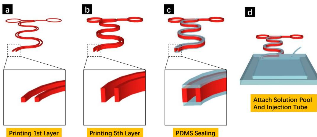
**Figure S1.** Schematic illustration of the manufacturing process of our capillary pressure sensor. (a) Printing 1st and (b) 5th layer directly on temper glass substrate; (c) Seal the top and bottom of the adjacent conductive electrodes to form the capillary conduction channel; (d) Attach solution pool and injection tube to complete the pressure sensor structure.
