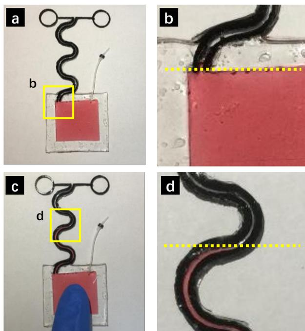
**Figure S3.** Photographs of the pressure sensor (a-b) without and (c-d) with external pressure. The liquid medium levels can be clearly viewed in the enlarged views.
